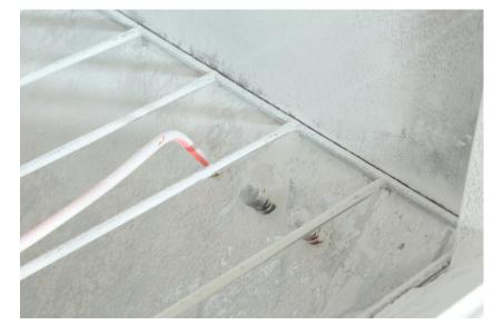
Dust collection section is located on bottom of test chamber.
